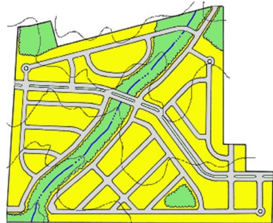
Figure 4.5.4.2 Fluid Grid Street Pattern
