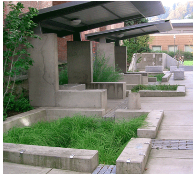
Figure 5.13.2.1 Urban Bioretention in Plazas
