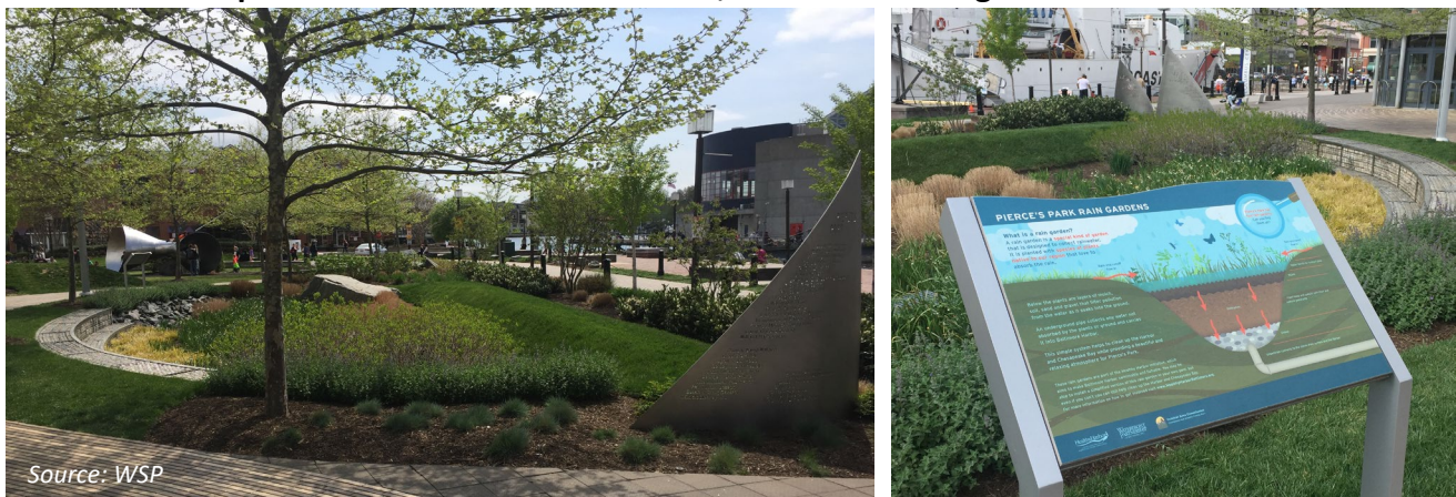
Figure 4.7.3.1 Example of a Pocket Park in Baltimore, MD with an Integrated Bioretention SCM
